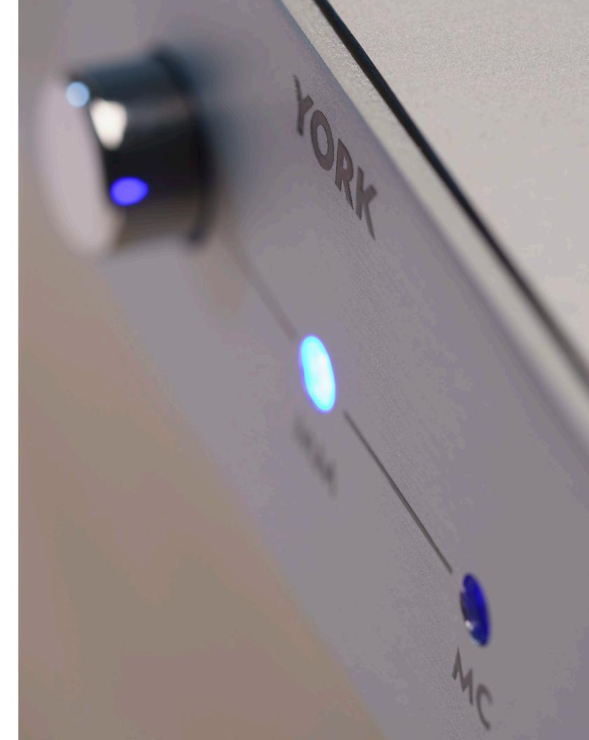
A pencil-sized tool is supplied for adjusting the input loading control. DIP switches on the underside of the unit allow for an adjustment of 0 pF to 470 pF capacitance for MM cartridges and 20 to 470 ohms impedance for MC carts. The RIAA curve is the only built-in EQ setting.
