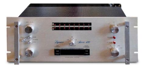
As high power was a fairly new concept for the time, one of the primary features of the Dynaco Stereo 400 was its Dynaguard power limiting system. This depended on the PC-29 Dynaguard board that held the protection circuit and a pair of 15 amp relays. This is probably the weakest link on what is otherwise a robust amplifier.
