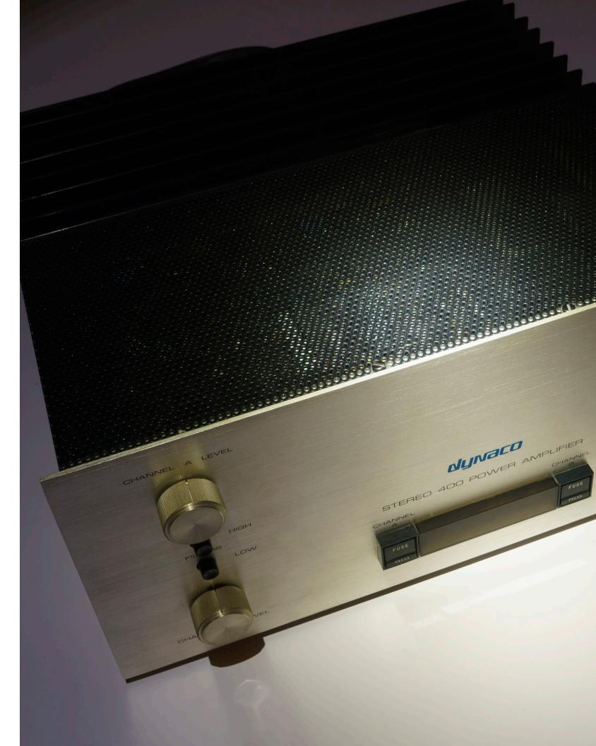
The Stereo 400 was pretty beefy, at 53 pounds. Stereo Review's Julian Hirsch bench tested the Stereo 400, measuring 248 Watts per channel into an 8-ohm load and 352 Watts per channel into 4-ohms. Nothing like the massive solid-state amps of today, doubling all the way down to 2-ohm loads, but still very powerful.
